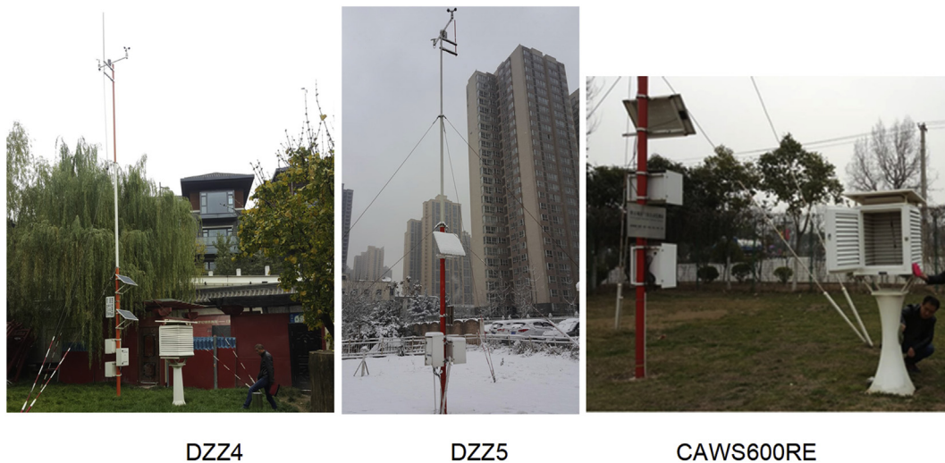
Fig. 4. Photos of three types of automatic stations in above meteorological stations.
