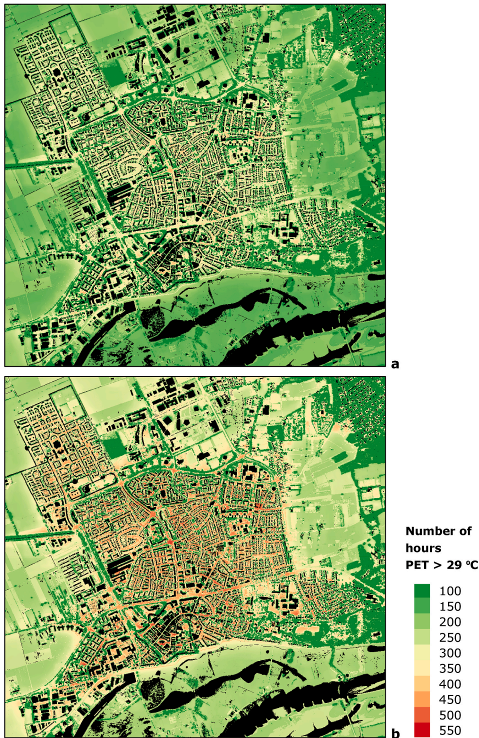
Fig. 10. Modelled number of hourly PET exceedances above 29 °C in 2013 for the current climate (a) and the W_H climate scenario (b) with the meteorology of the Herwijnen reference station.
